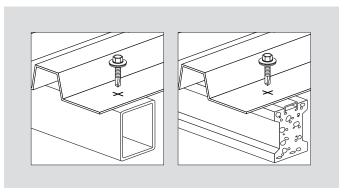
A2 stainless steel version, with hardened carbon steel drill point with fitted EPDM sealing washer
