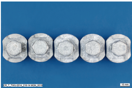
Fig. 19: Connector part with multilayer coating (organic flake topcoat) after ten weeks in the ISO 20340 test with UV radiation.
