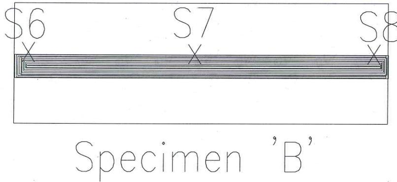
Figure 2 – Locations and reference number of thermocouples to monitor the temperature of unexposed surface of the specimen.
