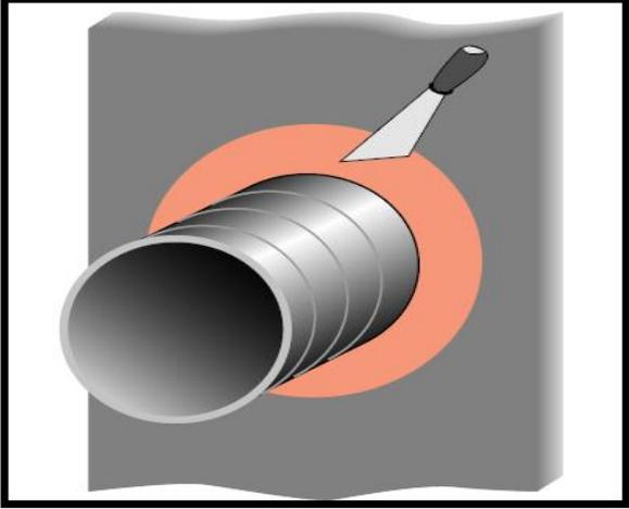
A 3D perspective illustration of a grey metal pipe protruding from a grey wall. An orange firestop sealant is applied around the pipe's circumference. A silver trowel with a black handle is shown smoothing the sealant. The sealant has a slightly textured, wet appearance.                                                                              |
