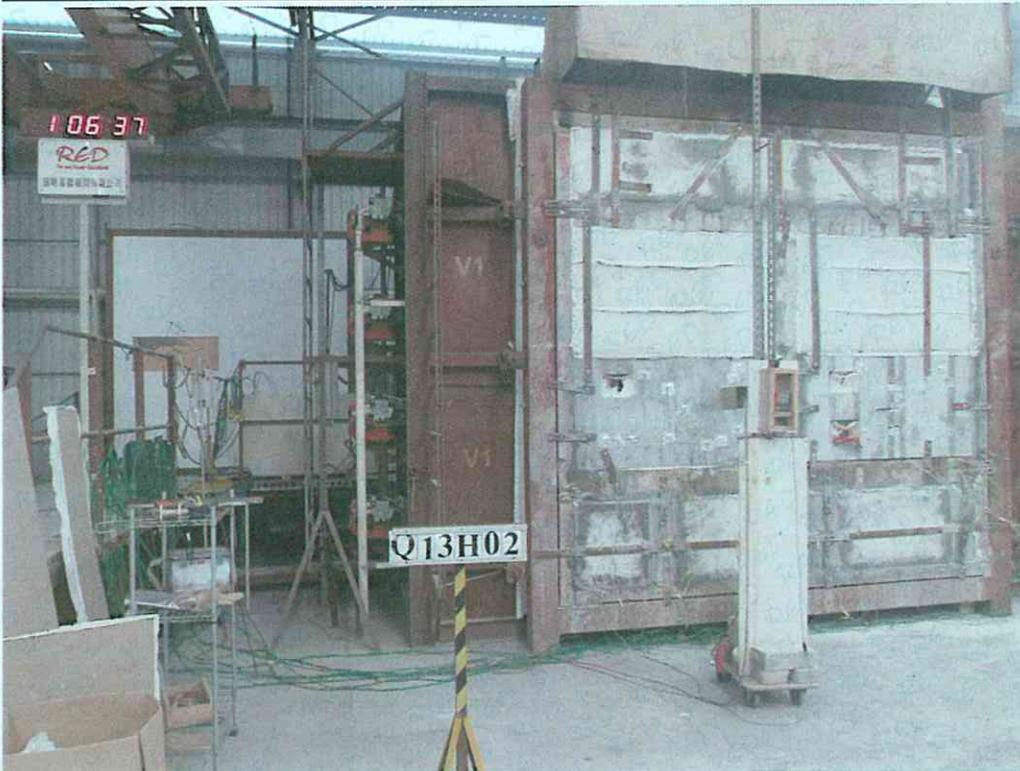
Photo 7 - The unexposed surfaces of the specimens after the test.
