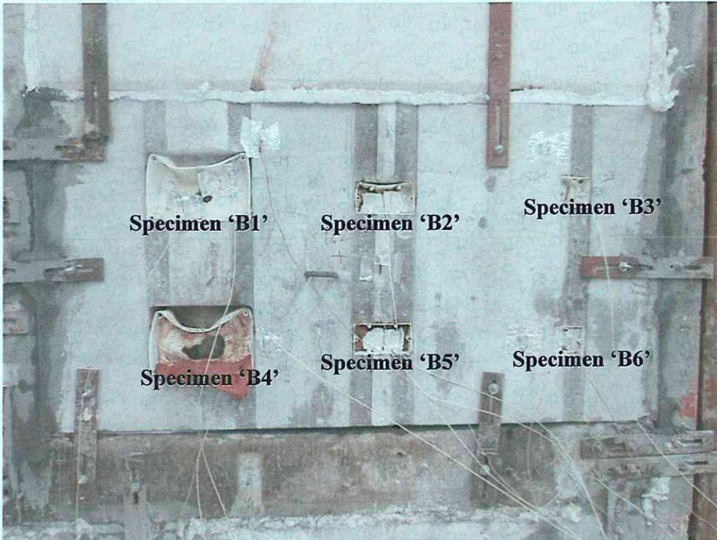
Photo 11 - The unexposed surface of the specimen 'B' after the test.
