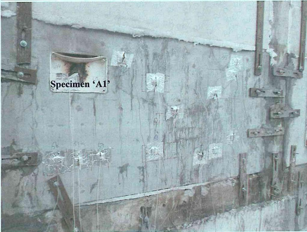
Photo 9 - The unexposed surface of the specimen 'A' after the test.
