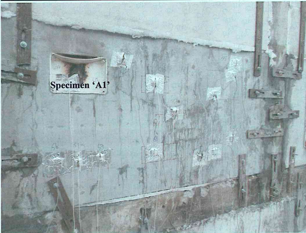
Photo 9 - The unexposed surface of the specimen 'A' after the test.
