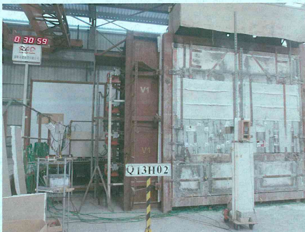
Photo 6 - The unexposed surfaces of the specimens after a heating period of 30 minutes.
