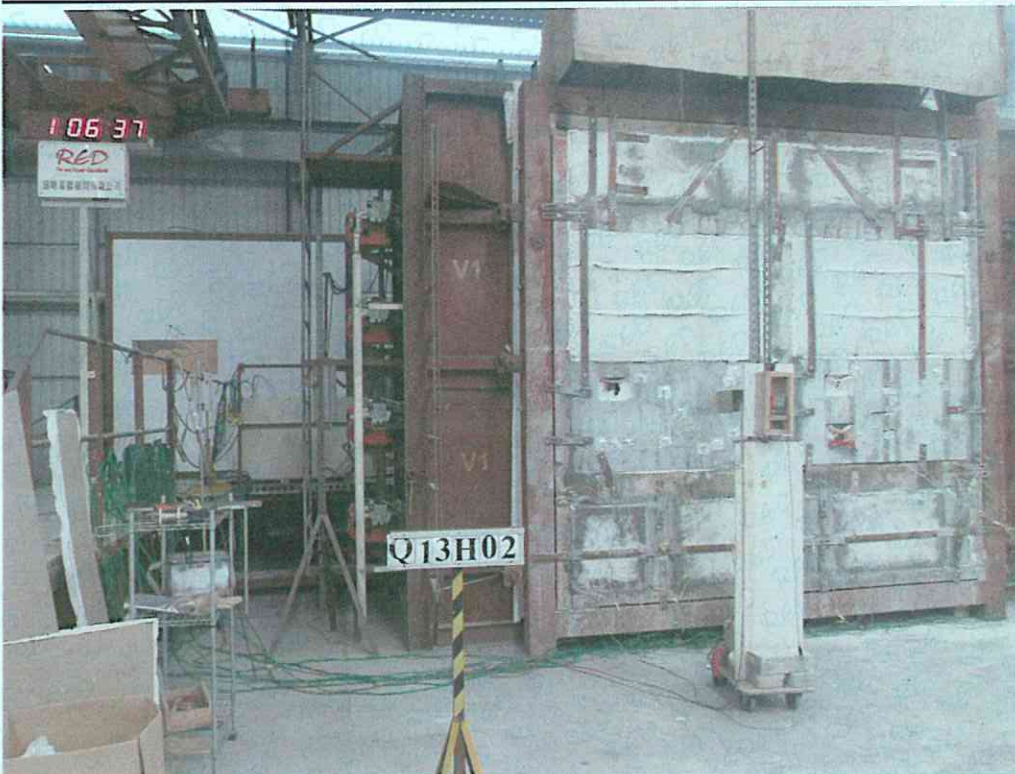
Photo 7 - The unexposed surfaces of the specimens after the test.
