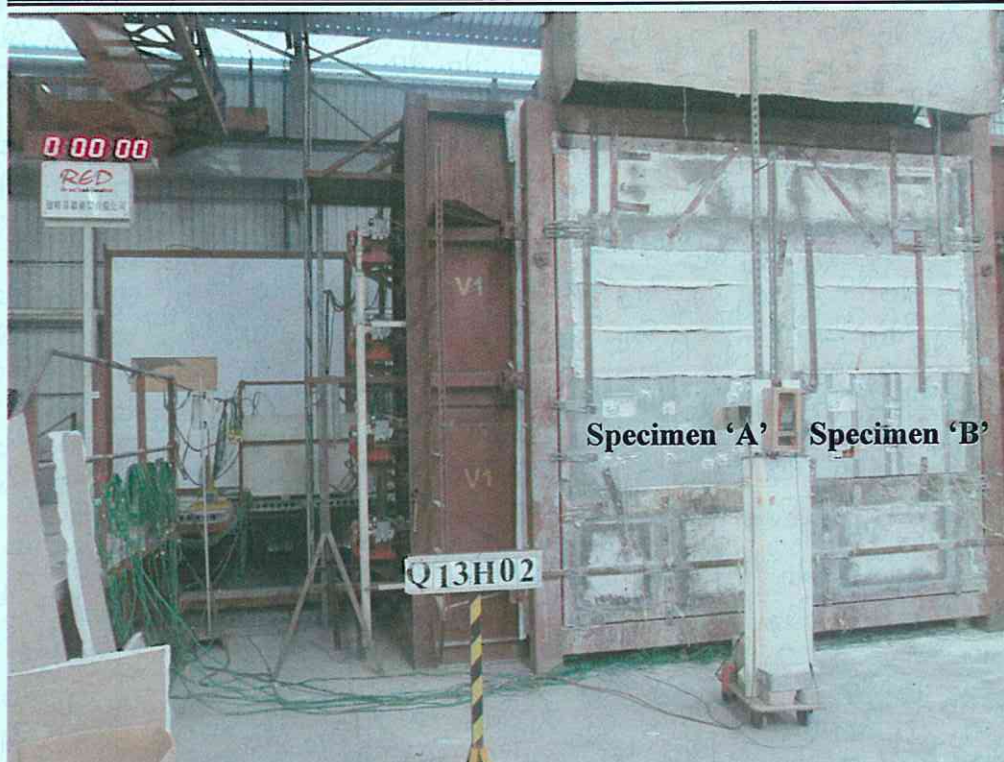
Photo 5 - The unexposed surfaces of the specimens before the test.
