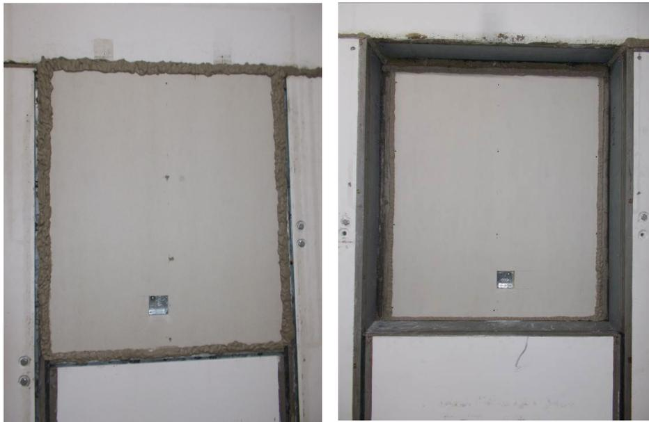
**Fig. 1** drywall insert unit with electrical box (from source room / receiving room)
