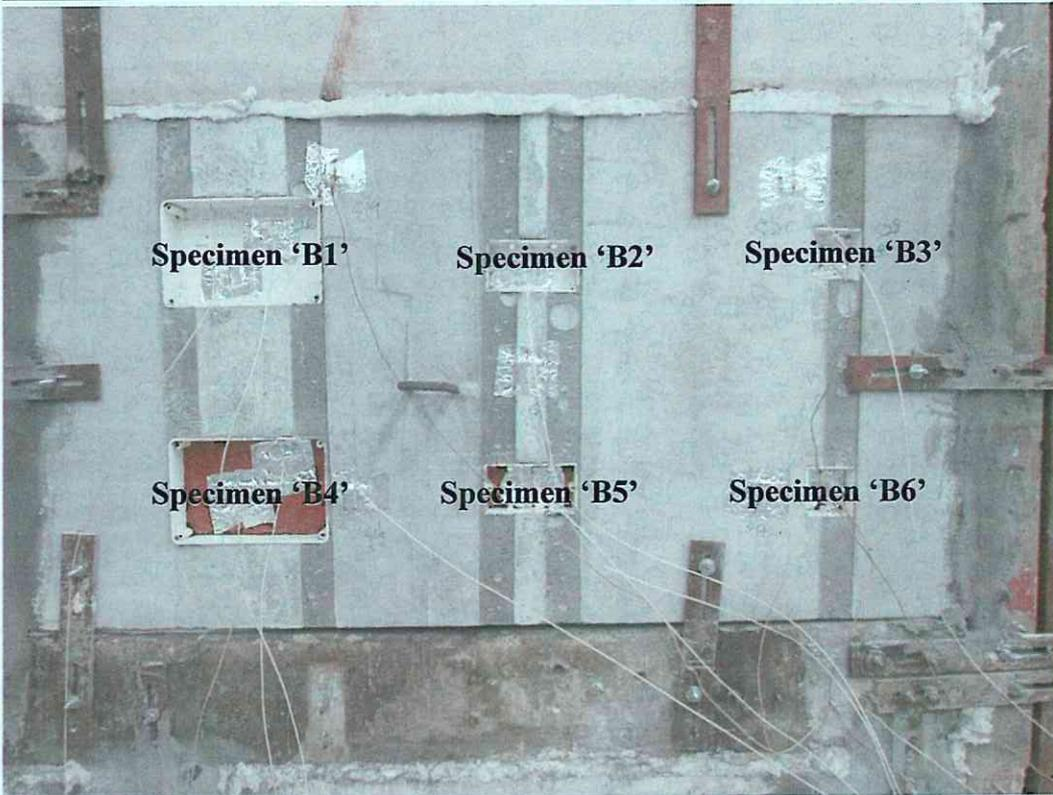
Photo 3 - The unexposed surface of the specimen 'B' before the test.
