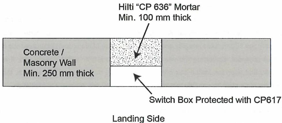
Figure 2: Illustration of the installation details of Hilti "CP636" firestop mortar for installation of switch box
