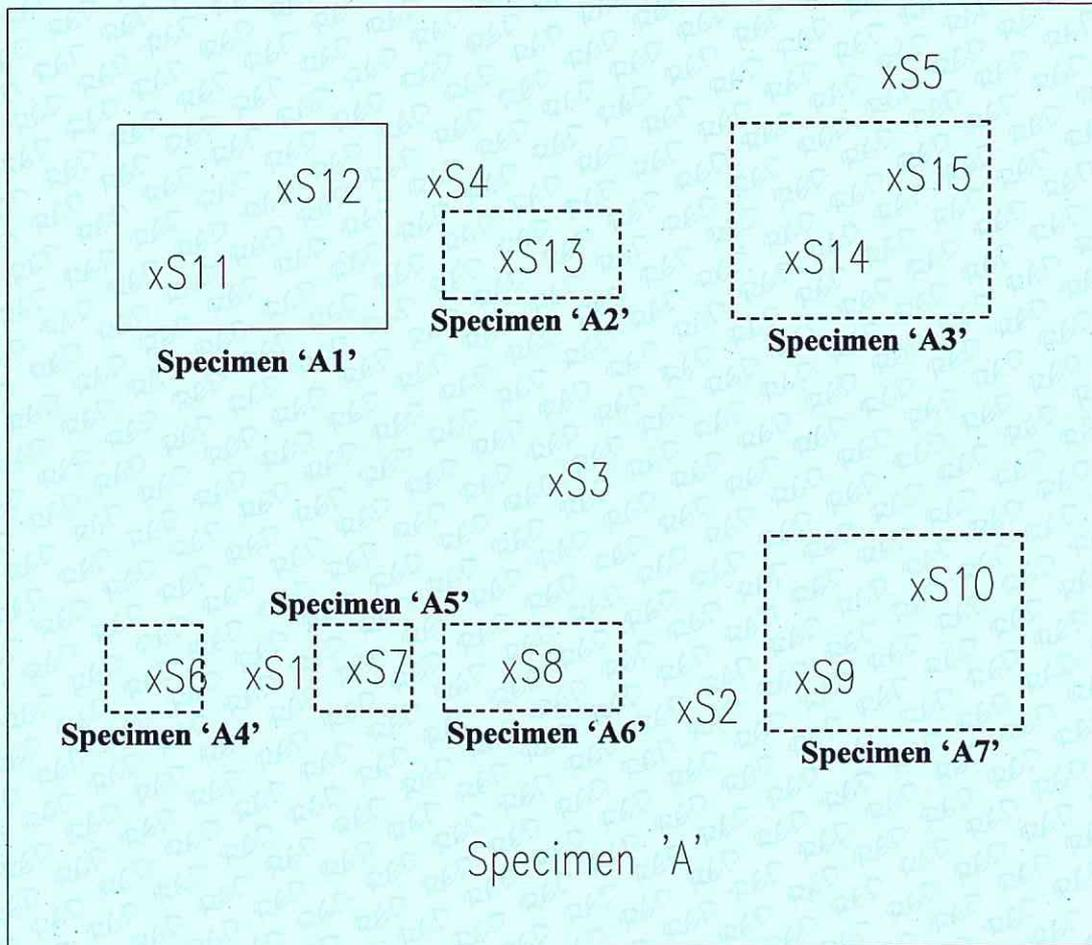
Figure 2 - Locations and reference numbers of thermocouples to monitor the temperature of unexposed surface of specimen 'A'. (This figure is not to scale)
