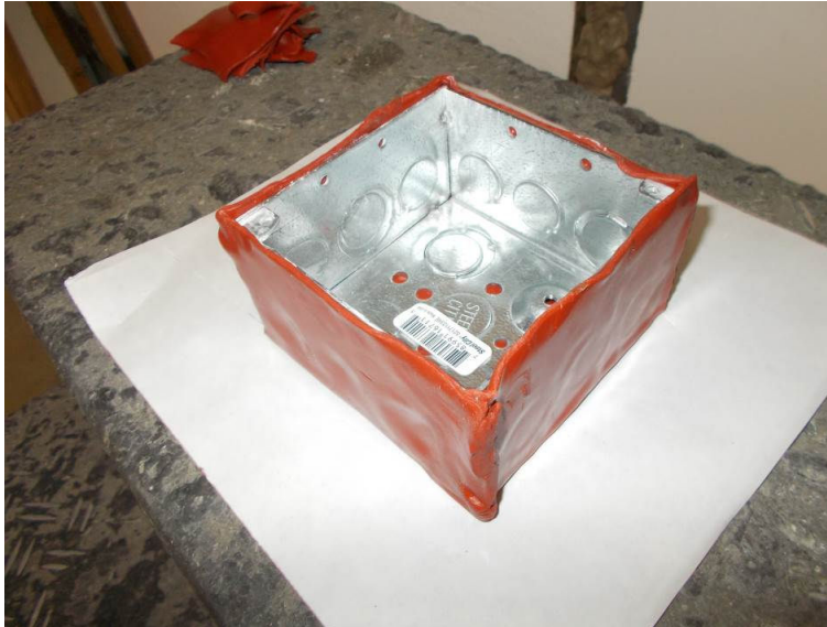
Fig. 3 Variant 4, metal box for electrical installation sealed with HILTI Putty Pad
