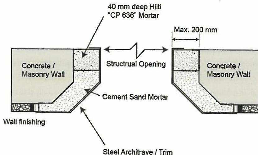
The Hilti "CP636" firestop mortar for use of lift-landing opening shall be capable to maintain the integrity performance for up to 120 minutes integrity performance when subjected to a test in accordance with BS 476: Part 20/22: 1987.
