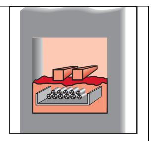
For maintenance reasons, a penetration seal could be permanently marked with an identification plate. In such a case, mark the identification plate and fasten it in a visible position next to the seal.
