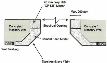
The Hilti "CP636" firestop mortar for use of lift-landing opening shall be capable to maintain the integrity performance for up to 120 minutes integrity performance when subjected to a test in accordance with BS 476: Part 20/22: 1987.
