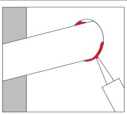
Close the CP 643N / CP 644 Firestop Collar. Place the CP 643N / CP 644 Firestop Collar around the plastic pipe and lock the closure by applying firm pressure until it latches.
