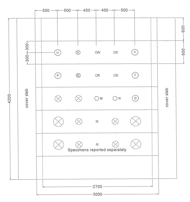
PLAN VIEW OF TEST ARRANGEMENT
