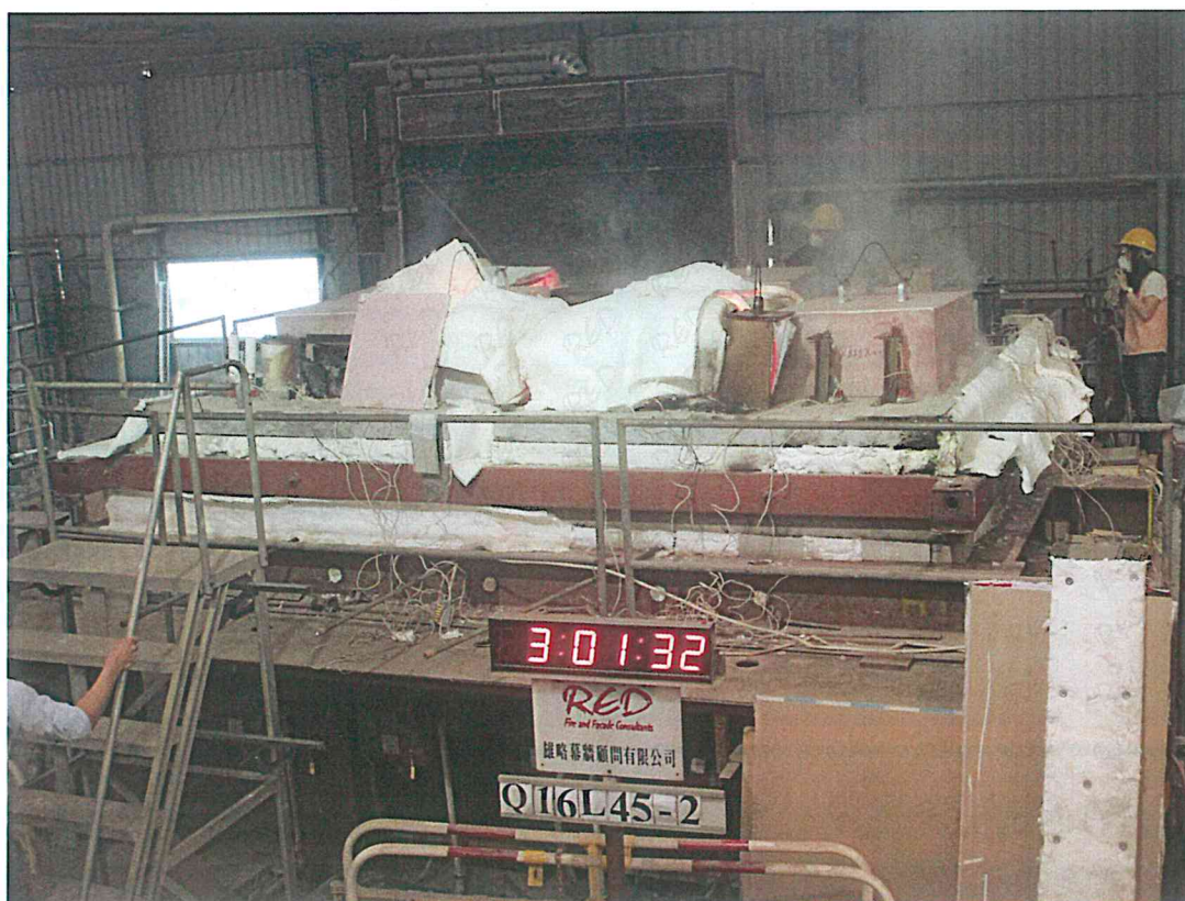
Photo 5: The unexposed face of the specimens after a heating period of 181 minutes.
