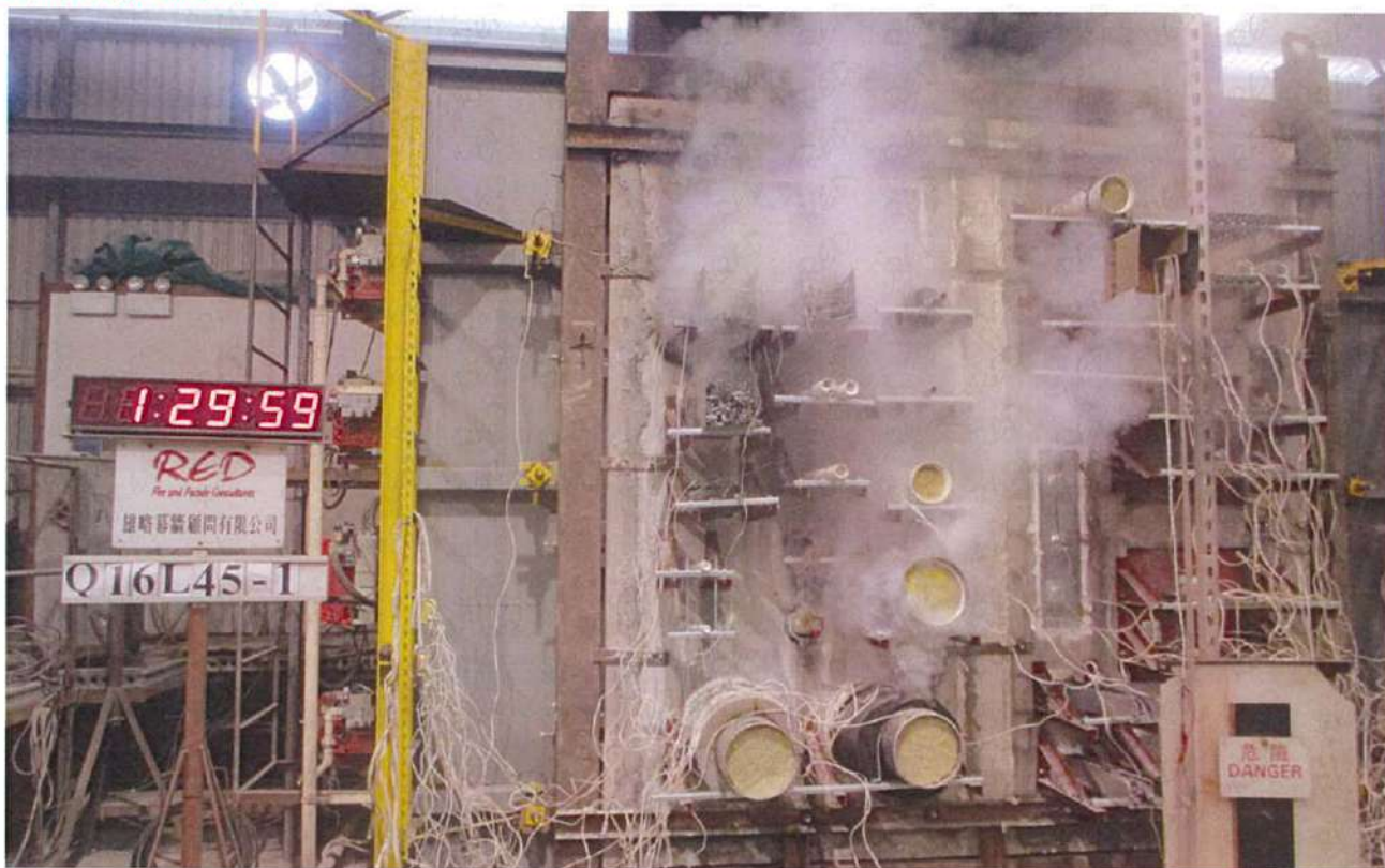
Photo 4: The unexposed face of the specimens after a heating period of 89 minutes.
