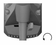
▶ Set the forward / reverse selector switch to forward or reverse rotation.
